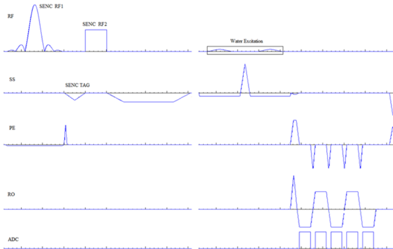
Fig. 1. Diagram of EPI-SENC pulse sequence with EPI factor of 5. Only one tuning is shown.
